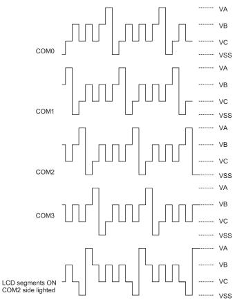
Note: 1/4 duty, 1/3 bias, C type: "VA" 3/2 VLCD, "VB" VLCD, "VC" 1/2 VLCD 1/4 duty, 1/3 bias, R type: "VA" VLCD, "VB" 2/3 VLCD, "VC" 1/3 VLCD
