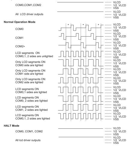
Note: "\*" Omit the COM2 signal, if the 1/2 duty LCD is used.
